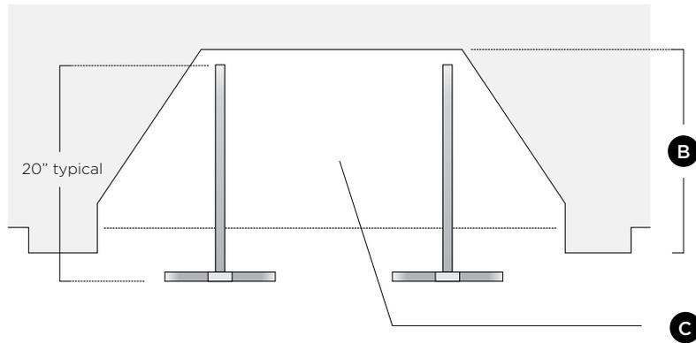
**C** Elevation or floor level inside firebox - typically will be flush with, or below, floor level at hearth.
