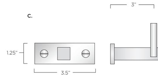
Note: center brackets are always available with either horizontal or vertical wall mounting plates and are often customized to accommodate site conditions
