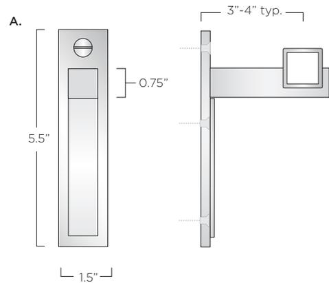
End Bracket Front / Side View / Double Rod
